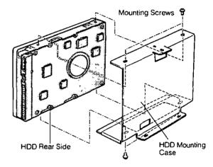
S Fix the HDD mounted on the Mounting Case onto Mounting Angle as indicated below.
