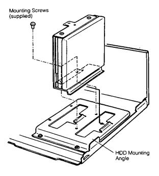
Tasten the Fixing Angle to the HDD Mounting Case and Chassis securely with three screws (provided).
