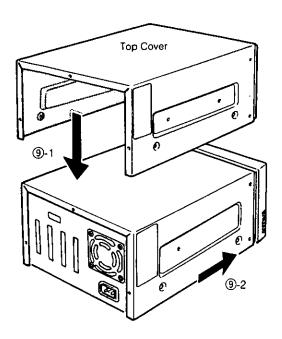
Fix the top cover on the HDD-BOX with 7 screws.
