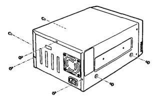
3 Slide the Top Cover in direction (3-1) and pull it upward (3-2).
